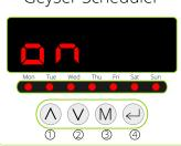
Pressing the mode button (3) will toggle between the 'off' for disable and 'on' for enble. Press enter (4) to save. This will enable or disable all schedules. If disabled, 'Soff' will appear when device is woken up.
