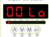
Cycle through each hour starting from '00', use or obuttons. Assign 'hi!/'lo' temperature using the mode button (3) to each hour.
