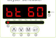
Press enter button (4) again to enter or change the boost temperature. Increase or decrease the boost temperature with  $\wedge$  (1) and  $\vee$  (2) buttons.
