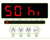
Setup high temperature 'hi'. Use © button (1) and @ button (2) to increase/decrease temperature.
