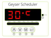
Press Enter button (4) to display current gevser temperature. LED (5) will be ON if the geyser is currently heating on schedule and FLASHING if
