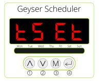
Press and hold the enter button (4) for 5 seconds to enter setup mode.
