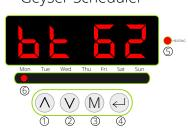
Press mode button (3) to select boost ON **BE OF** or boost OFF **BE OF** and then press the Enter button (4) to send the boost command. If on/off is not selected followed by Enter button, then boost command will not be sent. Default 45 C. Max 65°C, Min 20°C.
